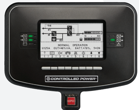
Monitor and Example Display Screen The display screen indicates "Normal Operation" (without alarms), with 40% output load and battery 70% charged. Numbers and icons are displayed to indicate each key's function.
