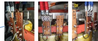
X1 to X4 (208 to 400V) X2 to X5 (208 to 400V) X3 to X6 (208 to 400V)
